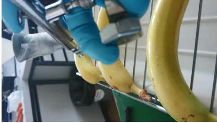
Atomizing Spray System; fibrillated carrot waste Cellulose in aqueous suspension
